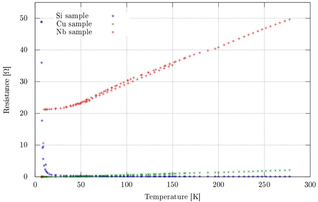
Figure 1: Resistance graph of all measured samples
