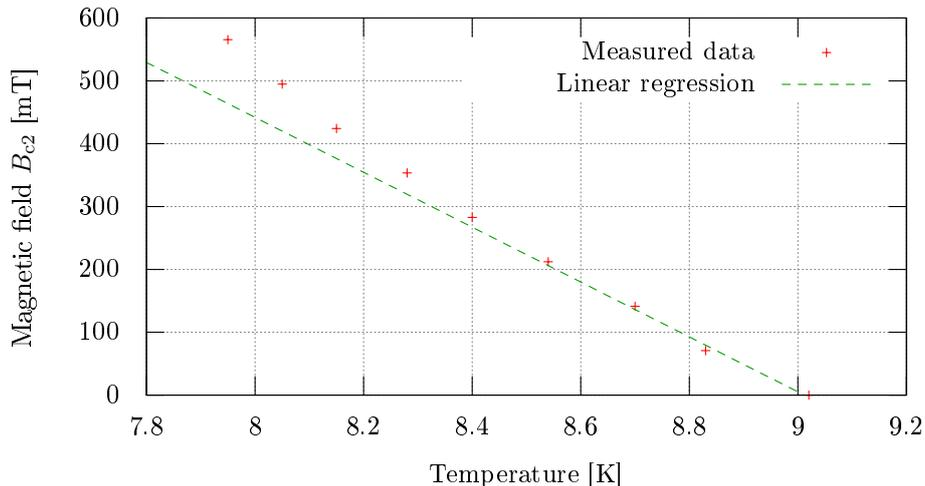
Figure 12: Measurement of critical magnetic field and temperature
