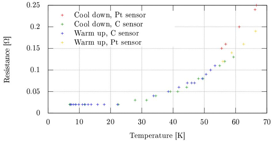
Figure 3: Resistance graph of Copper sample at lower temperatures
