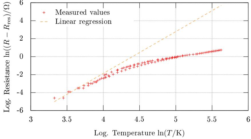
Figure 10: Double-logarithmic graph for copper
