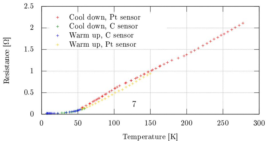
Figure 2: Resistance graph of Copper sample
