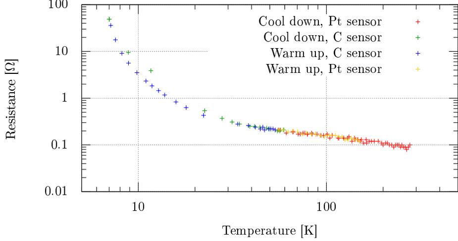
Figure 6: Resistance graph of Phosphorous doped Silicon sample
