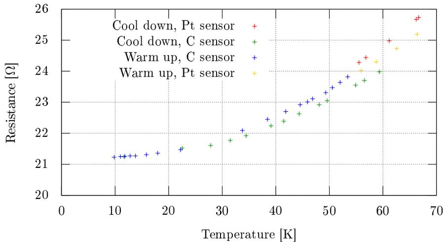
Figure 5: Resistance graph of Niobium sample at lower temperatures
