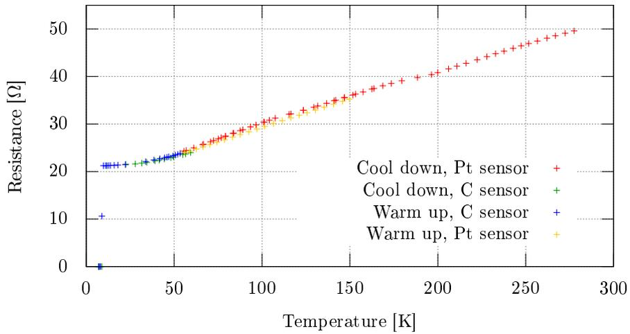
Figure 4: Resistance graph of Niobium sample
