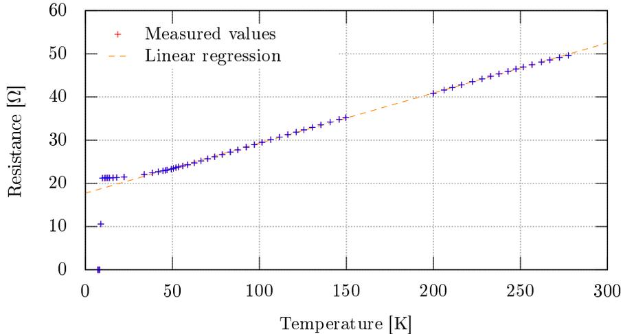
Figure 8: Linear regression of niobium at higher temperatures
