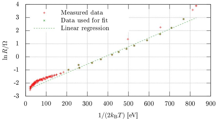
Figure 13: Activation energy of silicon
