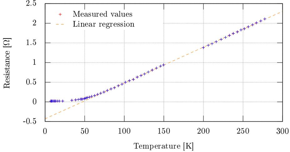
Figure 7: Linear regression of copper at higher temperatures
